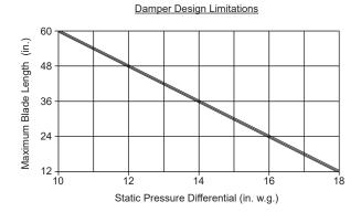
This damper's design at a length of 60" has a maximum allowable blade deflection of L / 360 for the static pressure indicated on the chart. At reduced blade lengths, higher static pressure limits can be attained without sacrificing damper operating performance characteristics.
