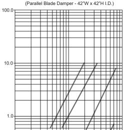
Pressure Drop vs. Duct Velocity
